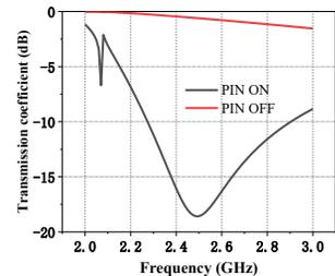
Simulated transmission coefficients of the switched FSS structure for ON and OFF states
