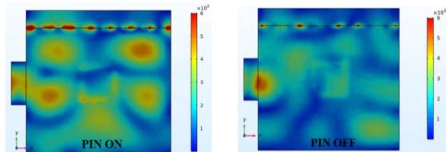
Simulated field distribution inside the cavity ( $z = 0$ ) for ON and OFF status
