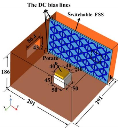
Geometry of the 3-D simulation model (unit: mm)
