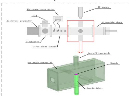
Fig. 1. Schematic of the microwave heating system
