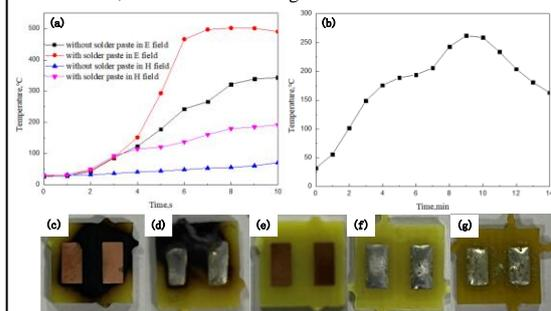
Fig. 2. Temperature rise curve of (a) conventional heating and (b) microwave heating, (c) the circuit without solder paste in E field, (d) the circuit with solder paste in E field, (e) the circuit without solder paste in H field, (f) the circuit with solder paste in H field and (g) the circuit with solder paste in conventional furnace
