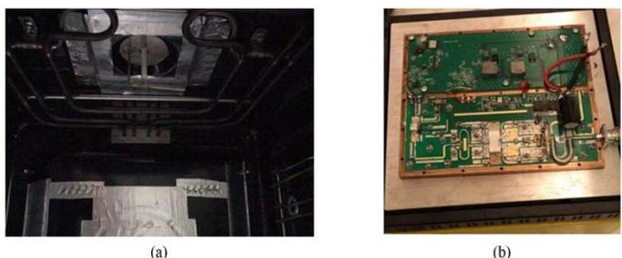
Fig. 1. The mounting position of the antenna inside the cavity and the actual solid-state source at 915MHz. (a) The installation position of the antenna inside the cavity; (b) The physical map of the 915MHz solid-state source.
