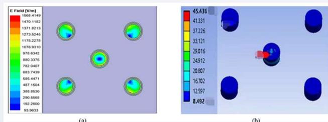
Fig. 3. Electric field distribution results and temperature distribution results on the surface of the water load. (a) The results of the electric field distribution on the surface of the water load; (b) The results of the temperature distribution of the water load.
