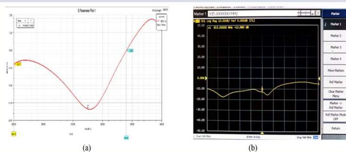
Fig. 2. Simulation results and measured results of the antenna. (a) Simulation results of the antenna; (b) Measured results of the antenna.
