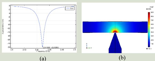
Figure 2. Numerical simulation results of open-end coaxial antenna resonator by 30-W microwave power at 2.45GHz.
