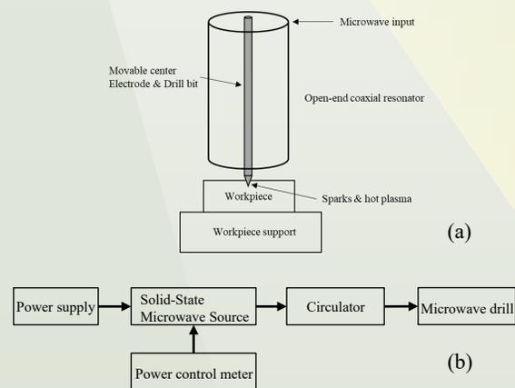
Figure 1. (a) Schematic diagram of the microwave drill
