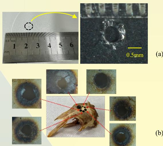
Figure 4. Microwave drilling pictures based on different materials
