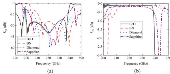
Fig. 2. Transmission characteristics of pillbox windows with different dielectric materials. (a)  $S_{11}$ ; (b)  $S_{21}$ .
