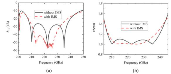
Fig. 3. Transmission characteristics of pillbox diamond windows without and with IMS. (a)  $S_{11}$ ; (b) VSWR.
