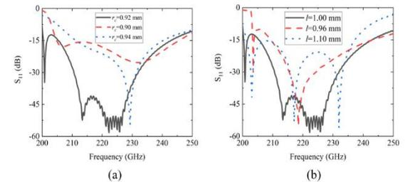
Fig. 4. Sensitivity of (a) Circular waveguide radius  $r_c$  and (b) its length  $l$ .
