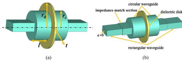
Fig. 1. The structures of the pillbox windows. (a) without and (b) with IMS.
